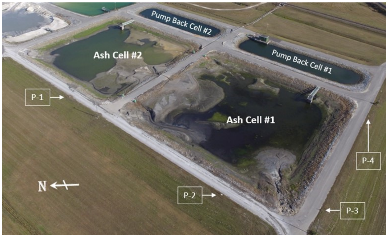
Figure 1. Layout of the CCR Surface Impoundment System and Adjacent Pump Back Ponds (IWCS 2016a)
